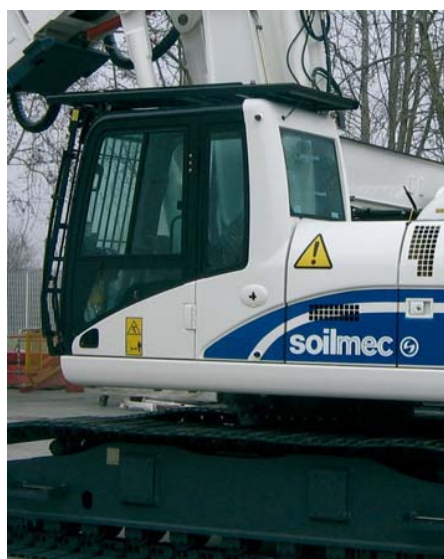
The new SR-40 is installed on new "Caterpillar" turret with easy access to any hydraulic and mechanical parts. New designed cabin allows better visibility and easier way of use.
